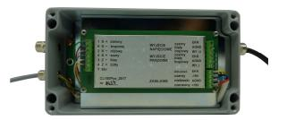
The CL 100P amplifier is designed for use with strain gauge sensors with 120÷1200  $\Omega$  full bridge. It is especially suitable for applications in a difficult climatic and mechanical environment. This amplifier is assigned for industrial use and other environments demanding high protection against dust, vibrations and humidity.
